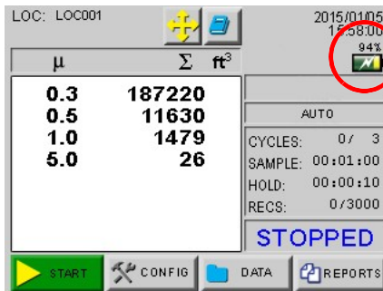
Figure 5-3 MAIN Screen - AC Operation
