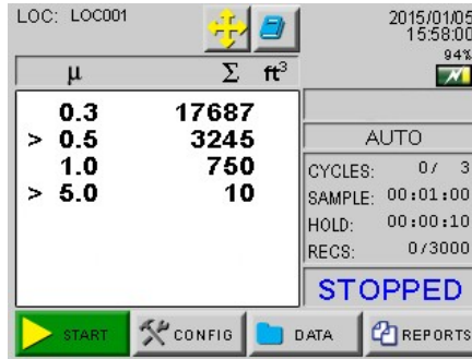
Figure 5-21 Channels Enabled for Alarming
