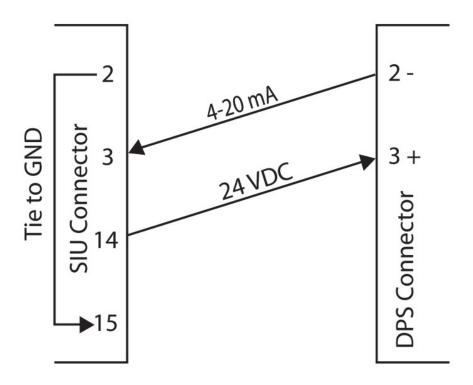
Figure 2-4 SIU DPS: Loop Power Wiring
