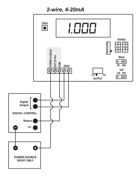
Figure 2-9 2-wire, 4-20mA System DP Wiring
