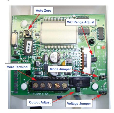
Figure 2-8 System DPS Adjustments
