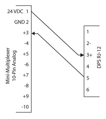
Figure 2-7 Mini-Multiplexer to DP Sensor Wiring
