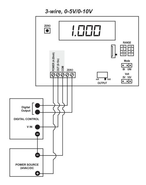
Figure 2-10 3-Wire, 0-5V/0-10V System DP Wiring
