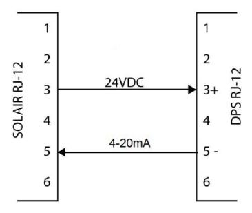
Figure 2-6 SOLAIR to DP Sensor Wiring
