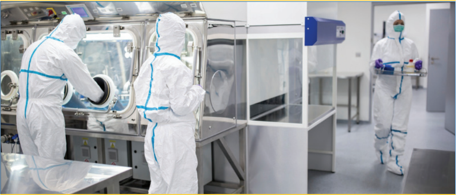
ISO 7 Pharmaceutical Cleanroom with separative devices
