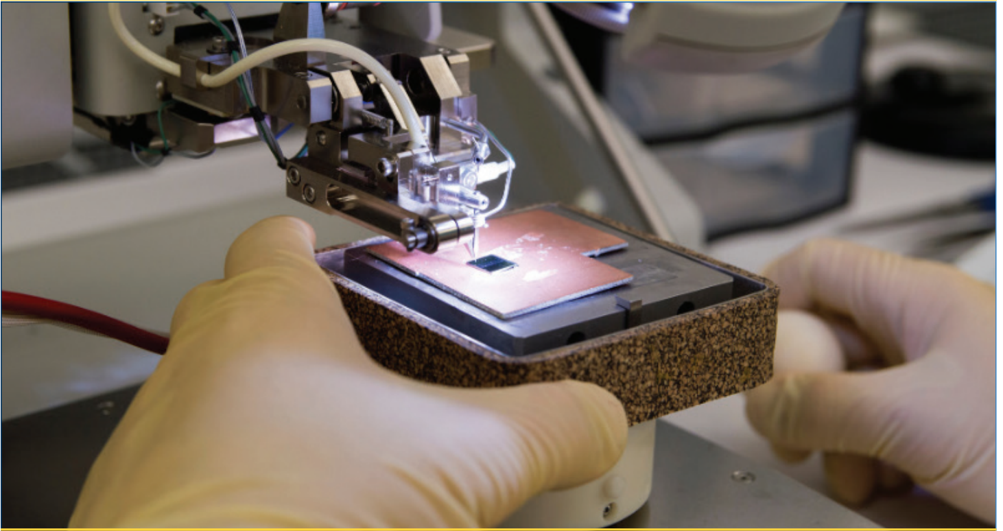
Semiconductor Wire bonding process in a Class 100 cleanroom
